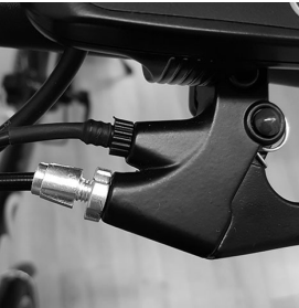
Applying the brakes activates the brake sensor which cuts the power to the motor.
