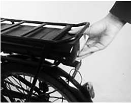
Withdrawing the battery from the case.
