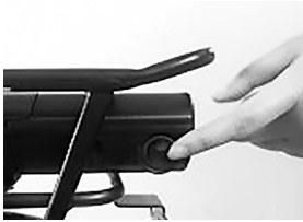
Switch battery ON
