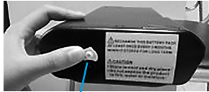
Battery charging connection point
