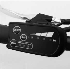
Check battery power indicator on the controller.
