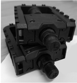
Stamped Crank ends 'L' and 'R'
